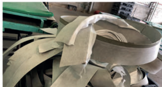
POST-CONSUMER: ALL TRIMMING PROCESS AND PRODUCTION REJECTS ARE REUSED TRIMMING OF THE PRODUCTION PROCESS AFTER GRINDING AND AGGLUTINATION
